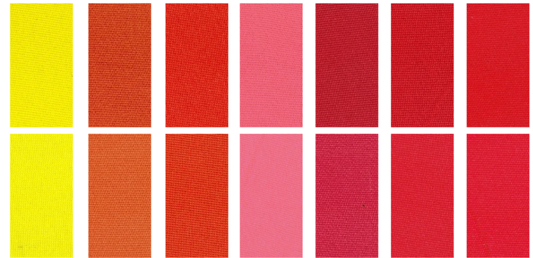
Yellow PS-6G 1.0% 2.0% Yellow Br. PS-2R 1.0% 2.0% Orange PS-3R 1.0% 2.0% Red PS-BEL 1.0% 2.0% Red PS-5B 1.0% 2.0% Red PS-RB 1.0% 2.0% Scarlet PS-2BL 1.0% 2.0%
