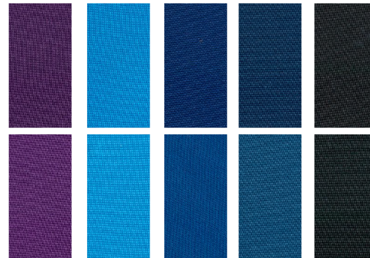
Violet PS-3B 1.0% 2.0% Brill Blue PS-BG 1.0% 2.0% Blue PS-RD 1.0% 2.0% Navy Blue PS-G 1.0% 2.0% Black PS-R 3.0% 5.0%
