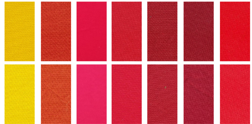
Yellow ME-4G 1.0% 2.0% Yellow Br. ME 1.0% 2.0% Red ME-FB 1.0% 2.0% Red ME-3B 1.0% 2.0% Red ME-4RB 1.0% 2.0% Rubine ME 1.0% 2.0% Scarlet ME-6S 1.0% 2.0%
